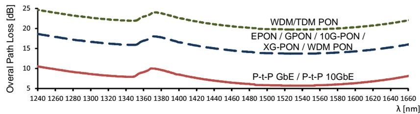
Fig. 4. Overall loss in the QKD signal path.
