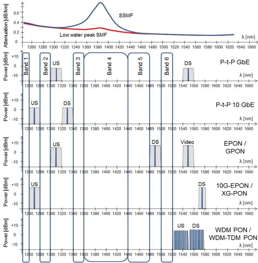
Fig. 2. Attenuation of optical fiber and wavelength plan for the considered optical access options. The marked wavelength regions (Band 1 - Band 6) are not used for classical communications and can thus be potentially used for QKD. Note that Band 4 can only be considered when using the low water peak fiber.
