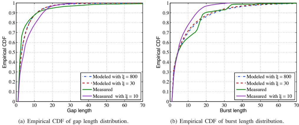
Fig. 3: Comparison of empirical CDFs of gap and burst lengths obtained from measured and modeled error patterns.
