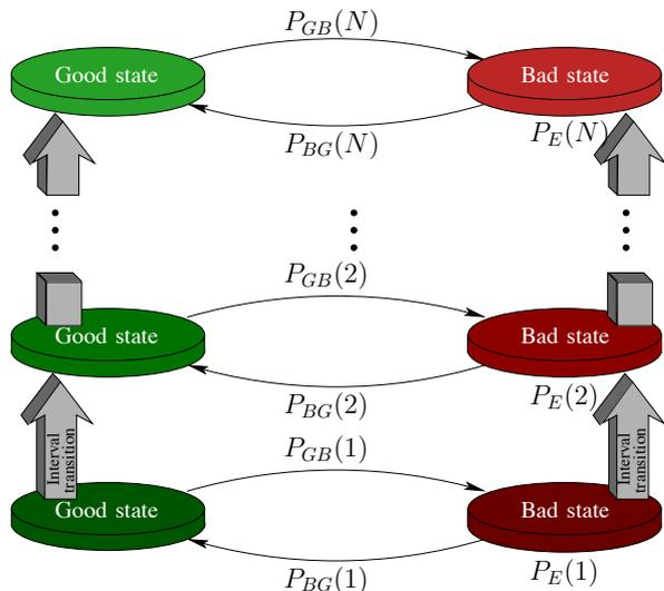
Fig. 2: Schematic illustration of range-dependent modified Gilbert model.
