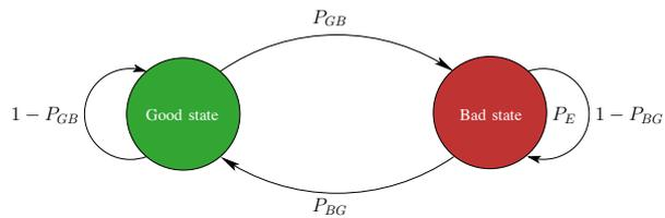
Fig. 1: Schematic illustration of Gilbert model.
