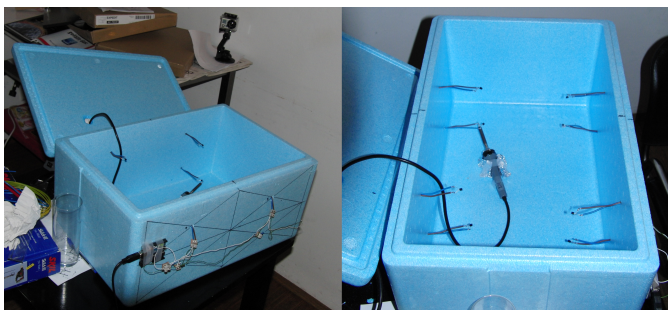
Fig. 7. Miniature Room Model Made of Polystyrene
