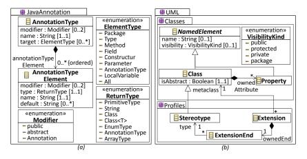
Fig. 2: Metamodel of Java Annotations and UML Profiles
