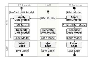
Fig. 4: Process for UML Profile Generation and their Application
