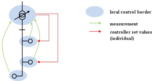
Figure 6: concept of stage 4 – “advanced control”
