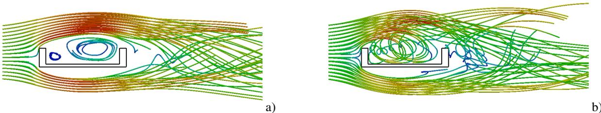
**Fig. 1:** Particle paths coloured by the velocity magnitude, simulation at  $Re = 2.45 \cdot 10^5$ . **a** R-flow pattern, **b** U-flow pattern.
