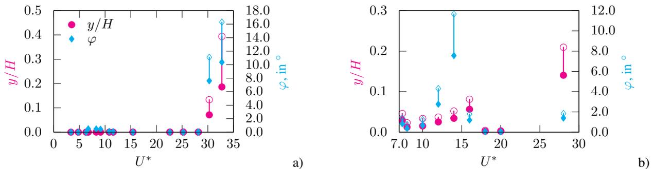
**Fig. 2:** Dimensionless heave and pitch amplitudes: R.M.S value (full symbol) and maximum value (open symbol) of a suitable time-interval: **a** Wind tunnel experiments,  $4.1 \cdot 10^4 < Re < 8.2 \cdot 10^4$ , **b** Simulation results  $Re = 2.45 \cdot 10^5$ .
