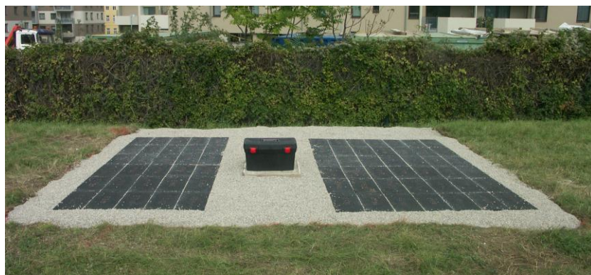
13 14 FIGURE 3 Photo of the Test Field with Winter Maintenance Section (left), Electric Cabinet (center) and 15 Section without Winter Maintenance (right)
