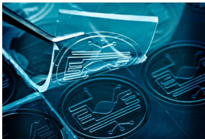
Figure 3.9: A microfluidic system being peeled out of its molding. Afterwards the PDMS can be placed on a sensor system to analyze the flowing samples [35].
