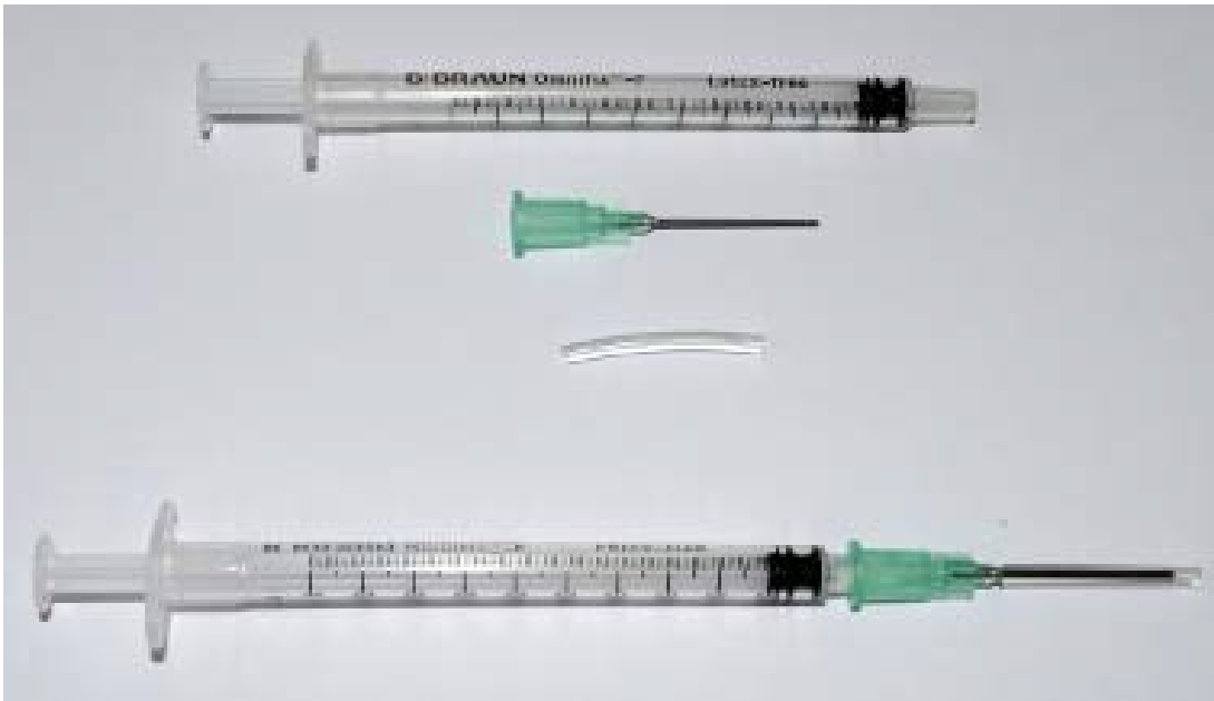
Figure 4.10: Shows the assembly of a syringe and a rubber tube which is used to bring the analyte sample inside the microfluidic channel. The rubber tube seals on the outlet of the channel and by applying a slight vacuum from the syringe the analyte sample will be sucked to its appropriate position inside the channel (i.e. the channel buffer).
