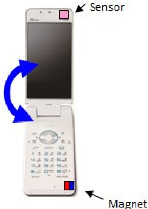
Figure 3.4: An AMR sensor used to detect the closure of the mobile screen.
