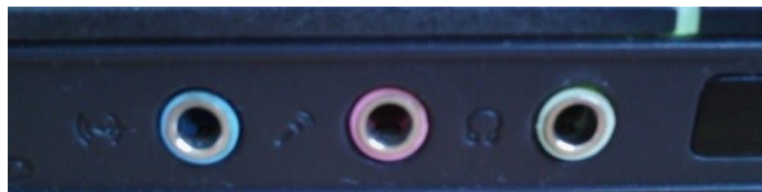
Figure 4.12: Typical soundcard channels left to right respectively (line-in, microphone and line-out).
