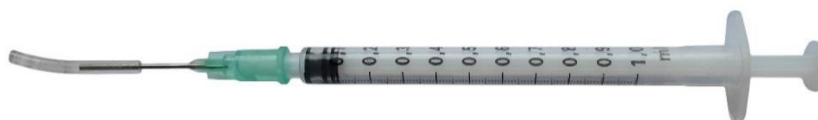
Figure 57: Syringe with needle and plastic tube as tip used for channel filling
