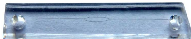
Figure 45: PDMS channel with inlet, outlet and a broader trapping channel area in the middle. The channel is in the \mu\text{m} range, while the overall PDMS is some mm thick.
