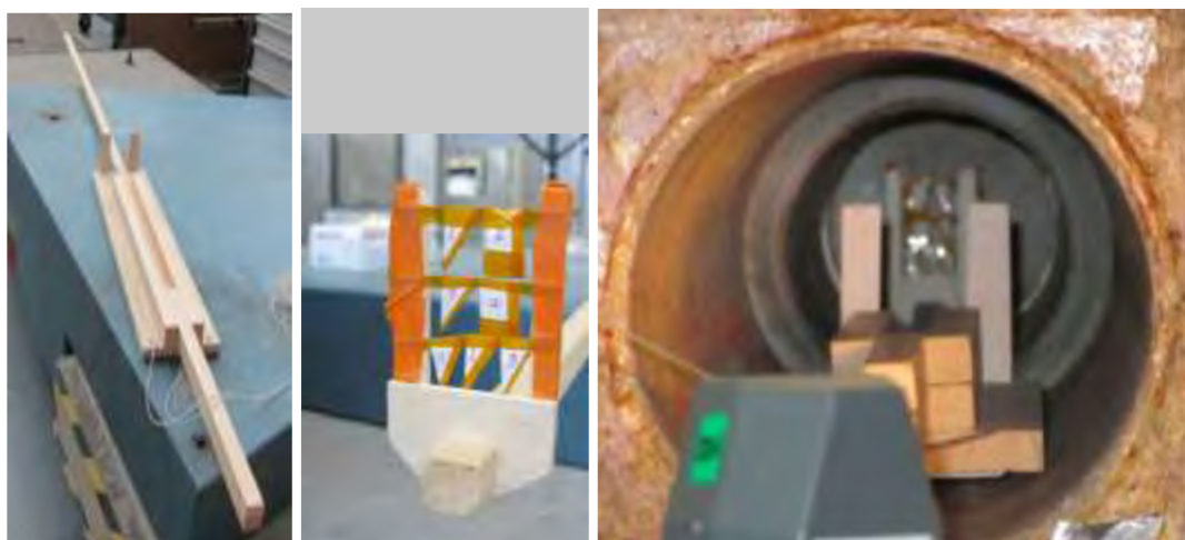
Figure 2: irradiation device used for foils irradiation in Beam Tube B and the positioning of the device inside the beam tube
