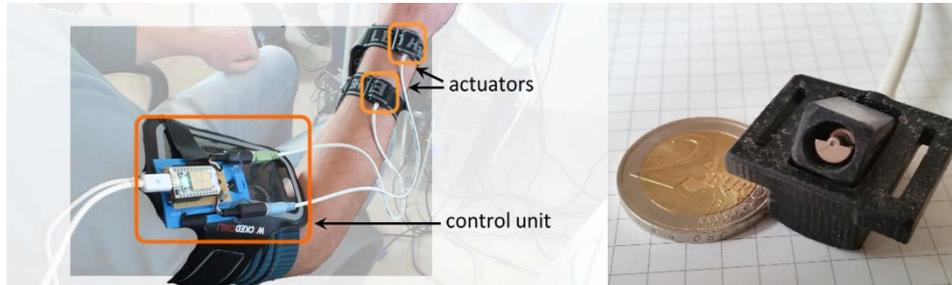
**Fig. 1.** Left: Apparatus employed during our experiment composed of a control unit driving two vibrotactile actuators controlled by a smartphone via a wireless connection. The two actuators were placed around the wrist at a distance of 10 cm. Right: Close-up of one actuator.
