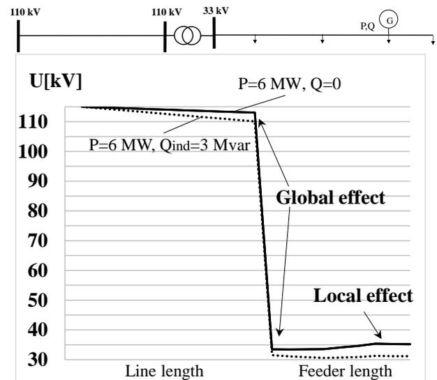
Fig. 3. Effects of the reactive power injection on the voltage profile.
