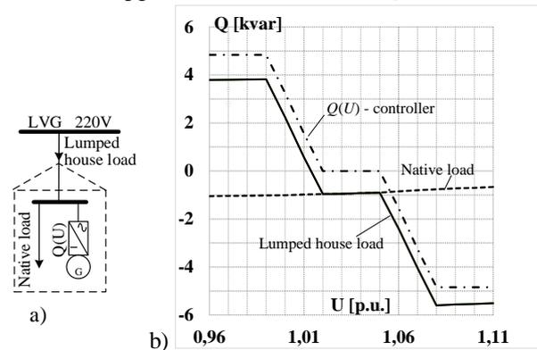
Fig. 5 Prosumer overview and its reactive power voltage sensitivity: a) Schematic representation b) Dependency of the reactive power from the voltage
