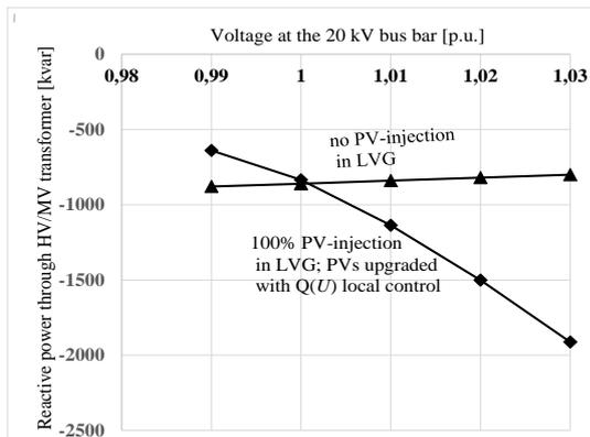
Fig. 6 Reactive power through HV/MV transformer for the maximum load with or without PV injection at LVG as a function of the voltages on the MV supply bus bar
