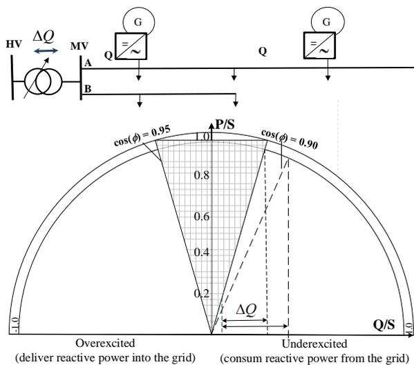
Fig. 4 PQ diagram of an inverter through which are connected PV and wind energy resources
