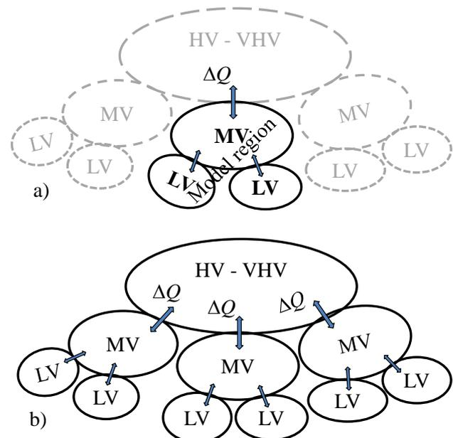
Fig. 1. General overview of the power grid: a) uncontrolled reactive power in the case of a typical model region; b) uncontrolled reactive power in the case of a large DG share on the whole power grid.
