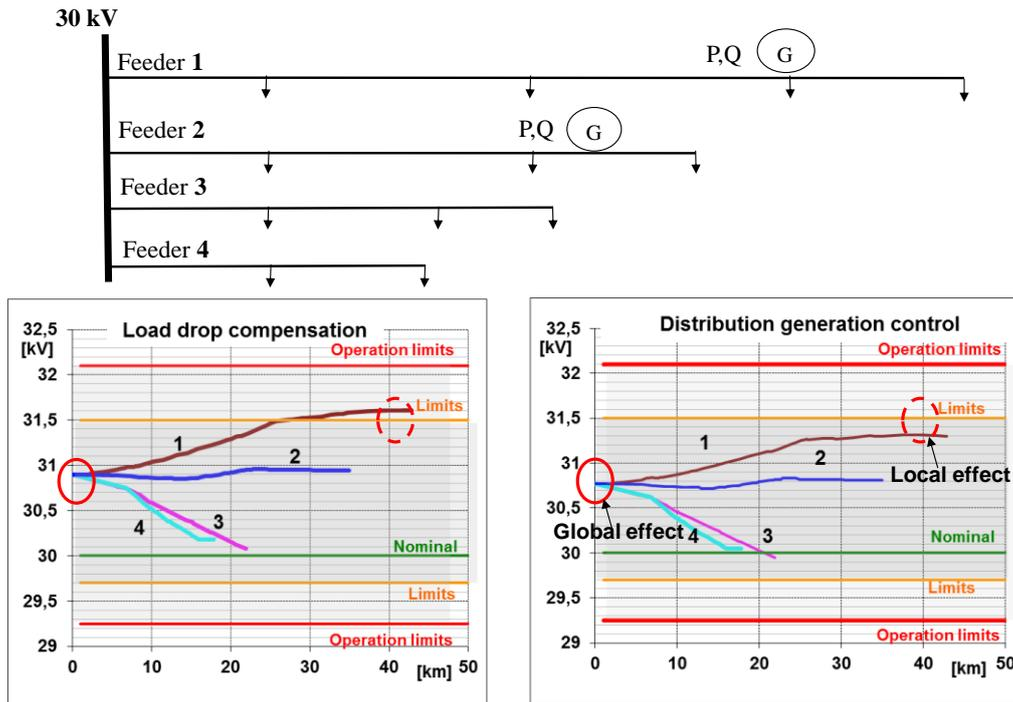
Fig. 2. Voltage profiles of 4 real feeders under: a) normal operation conditions and b) distribution generator control (source /2/)
