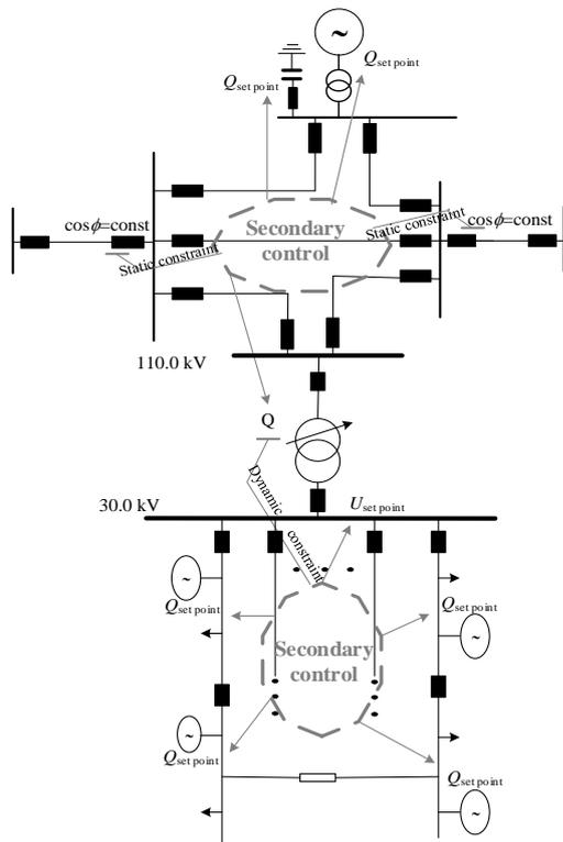
Fig. 8. Control schema for the coordinated operation of the medium and high voltage grid
