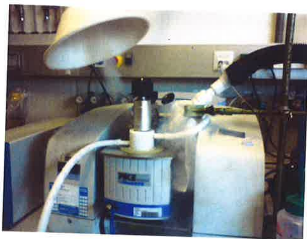
Figure 1. Variable temperature MIR/FIR-ATR unit
