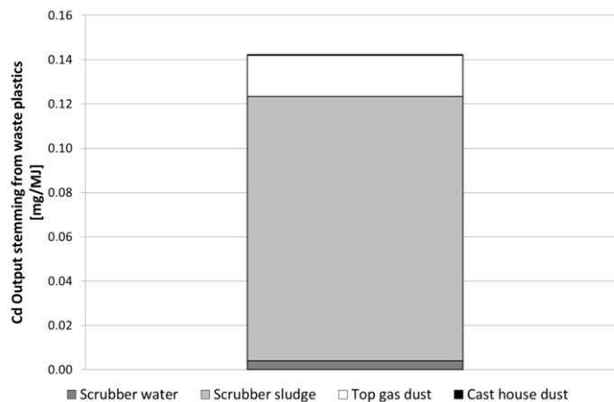
Figure 8: Specific Cd output for the HM production due to waste plastics utilization (given in [mg/MJ])
