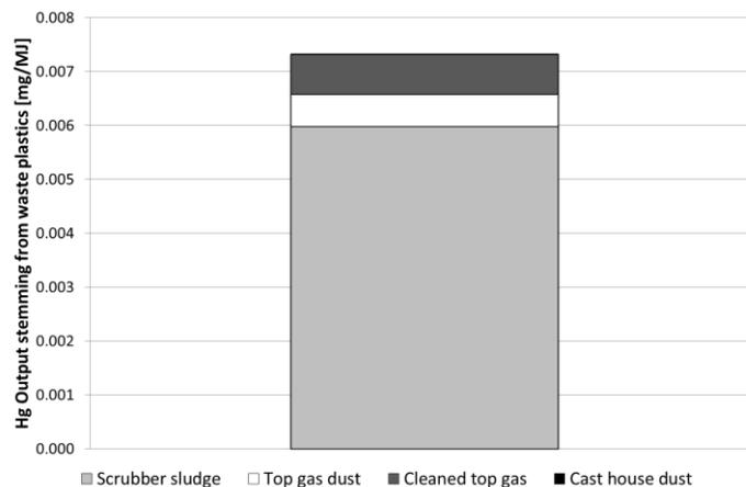
Figure 10: Specific Hg output for the HM production due to waste plastics utilization (given in [mg/MJ])
