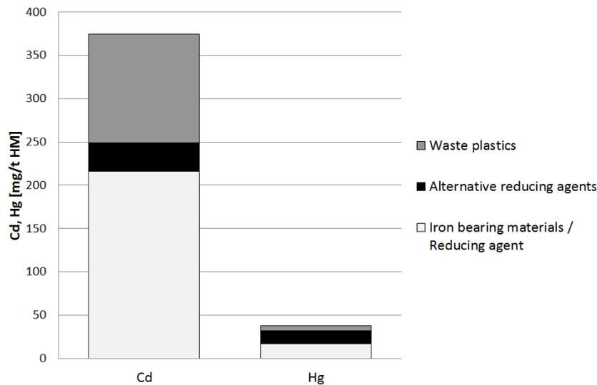
Figure 5: Cd (left) and Hg (right) input into HM production via different materials (given in [mg/t HM])
