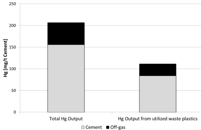
Figure 13: Hg output from the cement production process (left bar - total Hg output; right bar - Hg output due to waste plastics utilization) according to Lederer et al. (2015) given in [mg/t cement]
