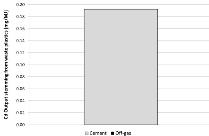
Figure 12: Specific Cd output from the cement production due to waste plastics utilization (given in [mg/MJ]) - according to Lederer et al. (2015)
