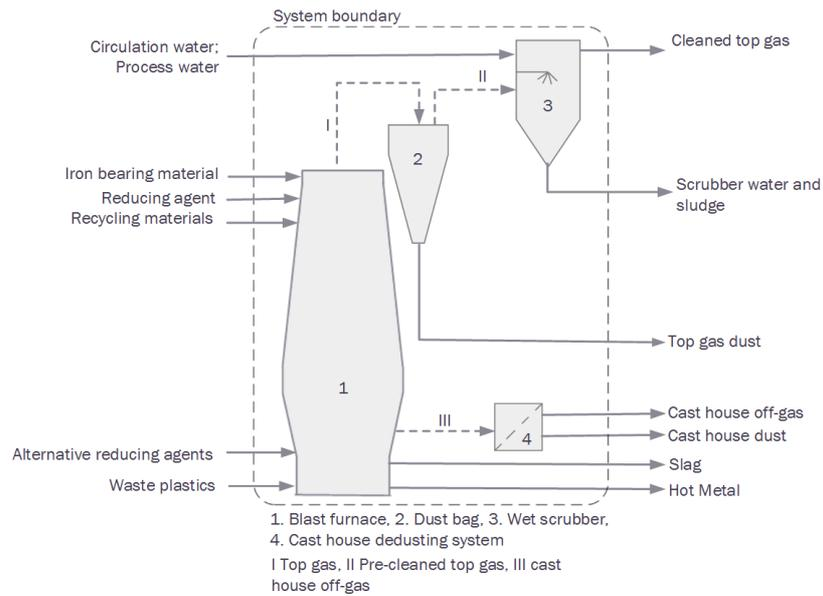
Figure 3: Blast furnace process model based on Trinkel et al. (2015)
