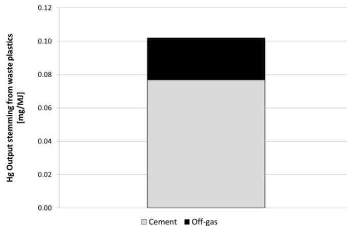
Figure 14: Specific Hg output from the cement production due to waste plastics utilization (given in [mg/MJ]) - according to Lederer et al. (2015)
