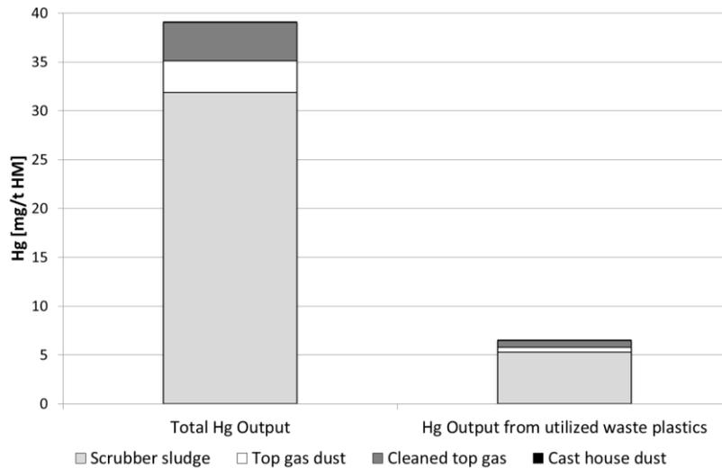
Figure 9: Specific Hg output from HM production process (left bar - total Hg output; right bar Hg output due to waste plastics utilization) given in [mg/t HM]
