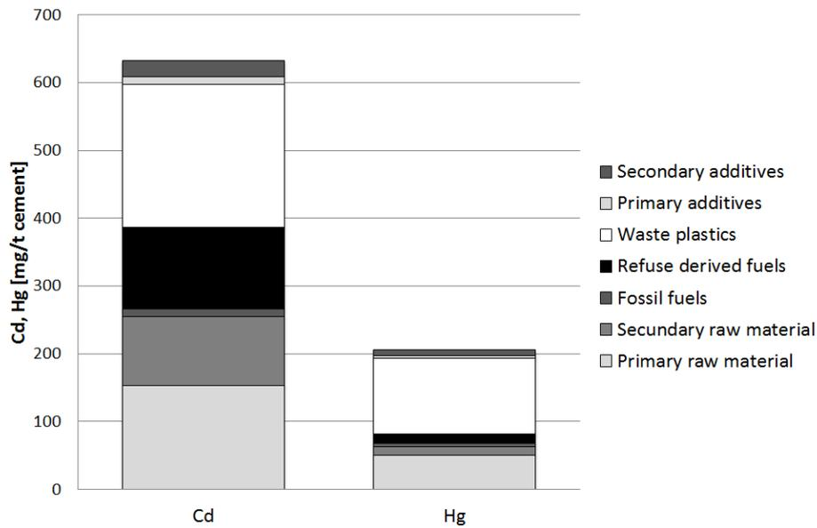
Figure 6: Cd (left) and Hg (right) input into the cement production process via different input materials (given in [mg/t cement]) - based on (Lederer et al., 2015)
