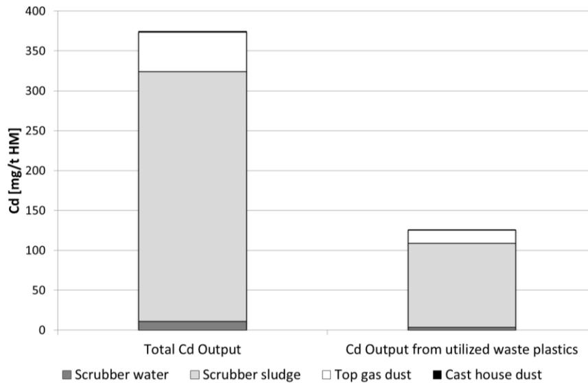
Figure 7: Specific Cd output from HM production process (left bar - total Cd output; right bar Cd output due to waste plastics utilization) given in [mg/t HM]
