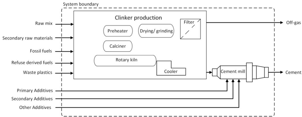
Figure 4: Modell of Cement industry based on Joint research centre (2013) and Lederer et al. (2015)
