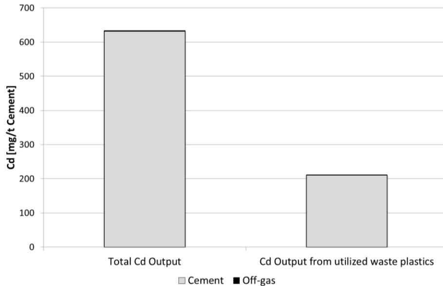
Figure 11: Cd output from the cement production process (left bar - total Cd output; right bar - Cd output due to waste plastics utilization) according to Lederer et al. (2015) given in [mg/t cement]
