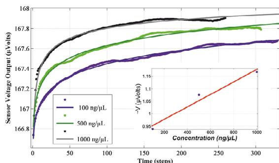
Figure 3. Change of the sensor's output voltage with the accumulation of the MNs on its surface versus time. Inset shows the linear ascent of  $\Delta V$  with concentration.
