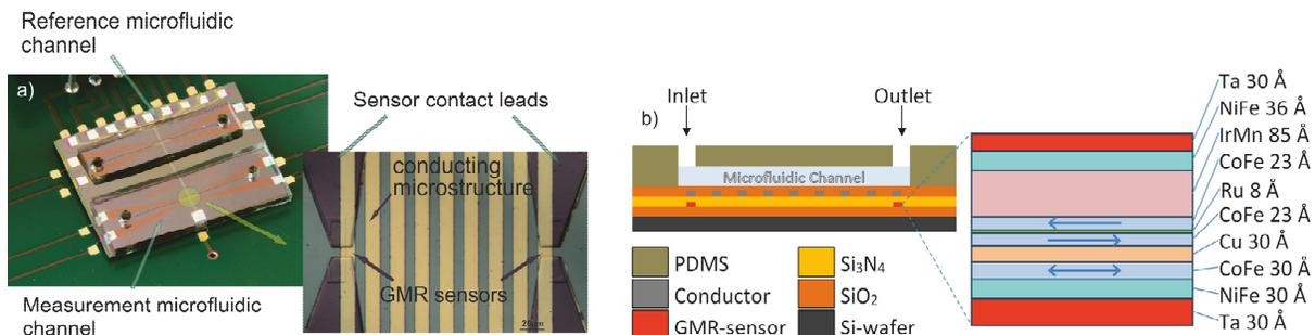
Figure 1: (a) Photograph of the proposed microfluidic chip mounted on a PCB board. In the accompanied microscope image the GMR sensors with their connecting leads and the micro conductors' area are shown. (b) Cross section of the chip with a detailed GMR, spin valve sensor element.
