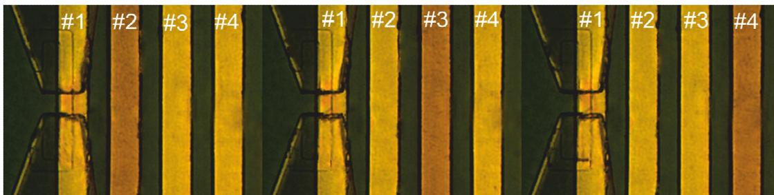
Figure 2: Sequential actuations of the MCs and manipulation of the MNs as a pre-concentration step. MNs are attracted to the current carrying MCs and are finally concentrated on MC #2.
