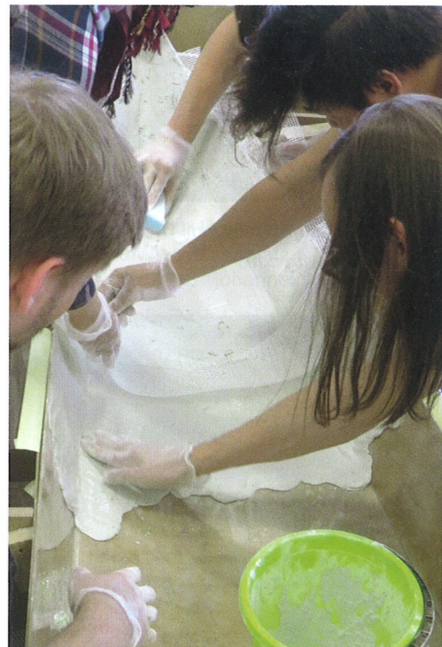
Abb. 5: Betonieren des Kanus Fig. 5: Placing of concrete of the canoe
