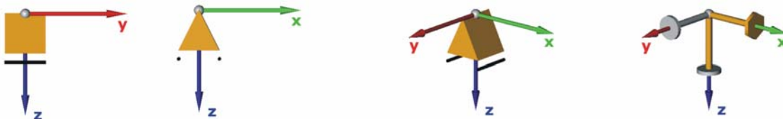
Figure 3: A complex support situation visualized as the bearing node of a structural behavior model – standard 2D view set and alternative 3D views (simplified and specialized proposals).
