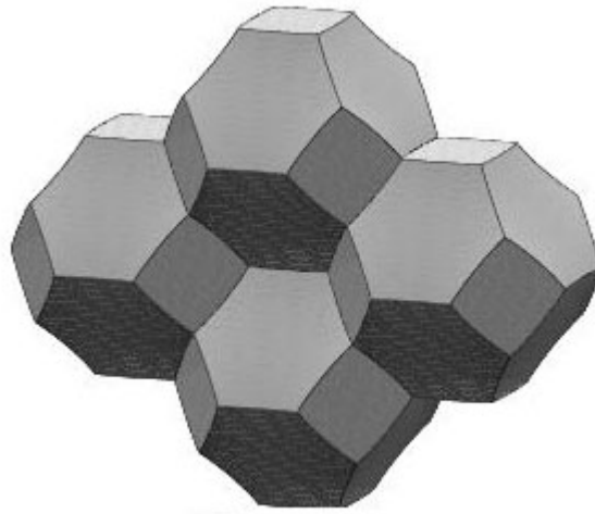
Figure 8: Orientation of Kelvin foam
