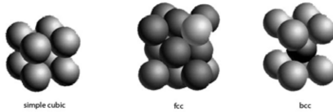
Figure 15: Packing types of foam models
