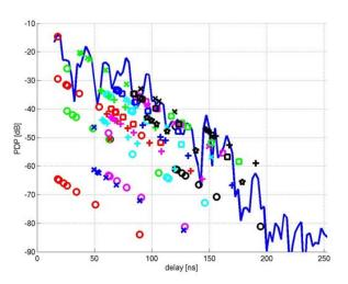
Figure 4: Exemplary instantaneous impulse response (blue line), and delay and power of all MPCs (colored markers).
