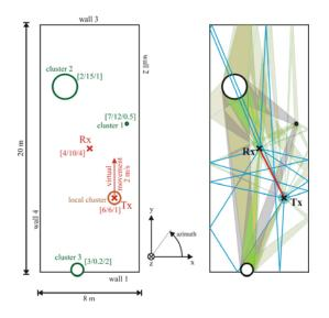
Figure 3: Room layout with physical clusters and link ends, and considered propagation paths.
