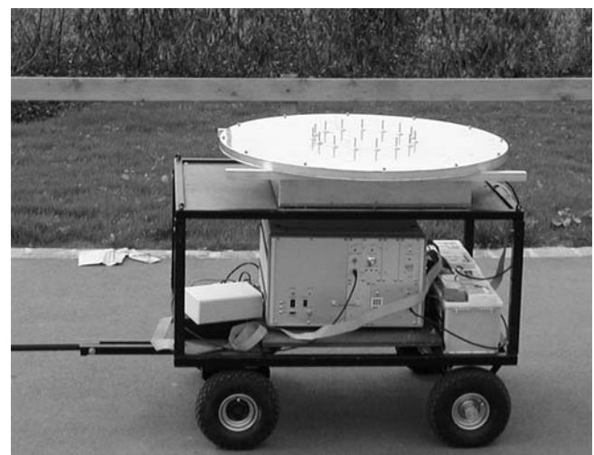
Fig. 5. 2 GHz transmitter on trolley, connected to 15 element circular antenna. Courtesy H. Hofstetter, ftw.
