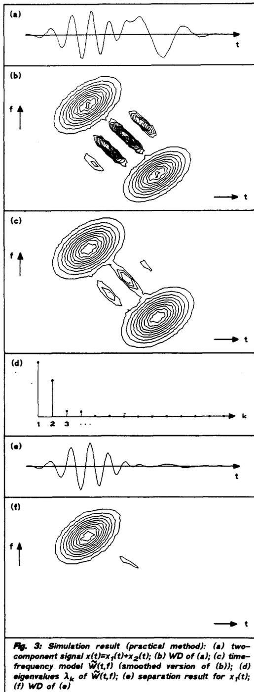
Fig. 3: Simulation result (practical method): (a) two-component signal  $x(t)=x_1(t)+x_2(t)$ ; (b) WD of (a); (c) time-frequency model  $\hat{W}(t,f)$  (smoothed version of (b)); (d) eigenvalues  $\lambda_k$  of  $\hat{W}(t,f)$ ; (e) separation result for  $x_1(t)$ ; (f) WD of (e)
