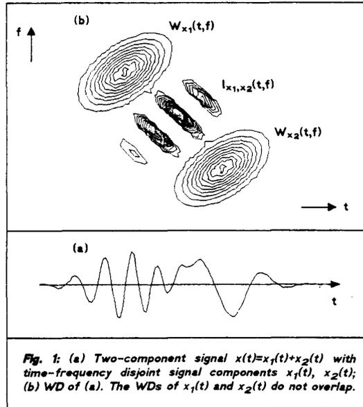
Fig. 1: (a) Two-component signal  $x(t)=x_1(t)+x_2(t)$  with time-frequency disjoint signal components  $x_1(t)$ ,  $x_2(t)$ ; (b) WD of (a). The WDs of  $x_1(t)$  and  $x_2(t)$  do not overlap.
