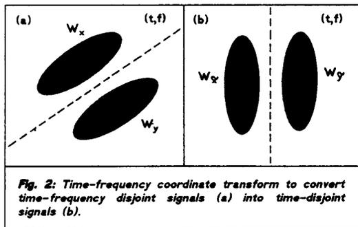
Fig. 2: Time-frequency coordinate transform to convert time-frequency disjoint signals (a) into time-disjoint signals (b).
