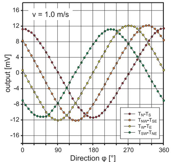
Fig. 4. Difference signals of opposed thermistors versus flow direction. The amplitude of the signals corresponds to a temperature rise of  $\approx 1.5 \text{ K}$ . The maximum sensitivity  $S = 152 \mu\text{V}/\text{deg}$  is obtained when the flow is perpendicular to the thermistor pair (zero-crossing of the curves).
