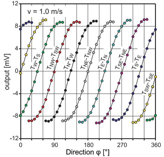
Fig. 7. Difference signals of thermistor pairs versus flow direction. The thermistors are arranged in a  $90^\circ$  angle around the heater. The maximum sensitivity  $S = 225 \mu\text{V}/\text{deg}$ .
