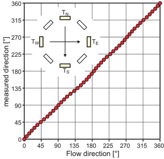
Fig. 5. Measured direction versus flow direction determined by Eq. (1).  $v = 1$  m/s.
