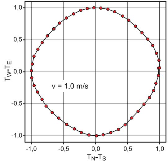
Fig. 6. Example of normalized difference signals of two perpendicular thermistor pairs
