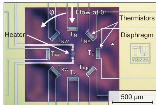
Fig. 1. Photomicrograph of the micromachined flow sensor.  $\varphi$  denotes the direction of the flow with respect to the N-S-direction. The different shading of diaphragm and leads is caused by the buckling of the diaphragm.
