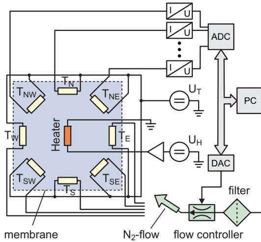
Fig. 2. Schematic measurement setup.  $T_N, T_{NE}, \dots, T_{NW}$  ... thermistors,  $U_N$  ... thermistor voltage,  $U_H$  ... heater voltage.
