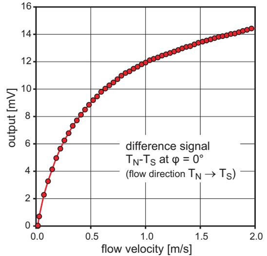
Fig. 3. Difference signal of a pair of diametrically opposed thermistors ( $U_{T_N} - U_{T_S}$ ) versus flow velocity. The channel is oriented in parallel to the connecting line of the thermistors.
