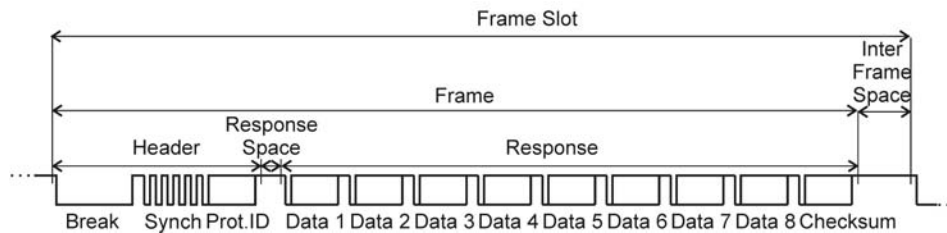
Figure 2.5: Structure of a LIN Frame[LIN03]
