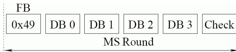
Figure 2.13: Structure of a TTP/A Master – Slave Round[EHK + 02]
