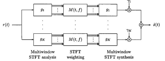
Fig. 3. Multiwindow STFT implementation of the Wiener filter.
