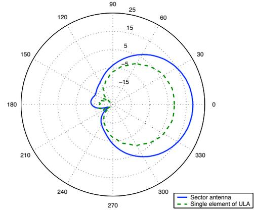
Fig. 2. Antenna pattern of the sector antenna and of a single element of the ULA used for beam switching. Radial unit is dB.
