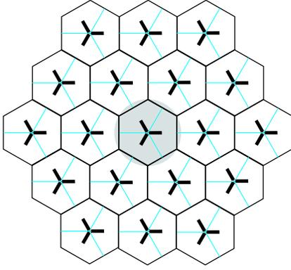
Fig. 1. Simulation area with 19 3-sectored base station sites
