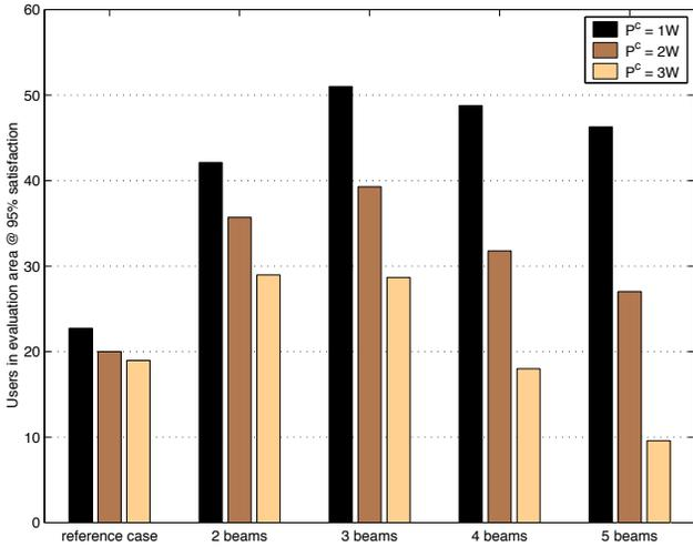
Fig. 3. Average number of users (95% satisfaction) for various base station configurations
