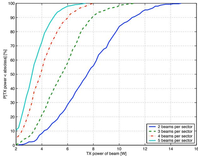
Fig. 5. Cdf of the transmitted power per beam for various beam switching schemes with  $P^c=2W$  and a load corresponding to 95% satisfied users (50 snapshots)
