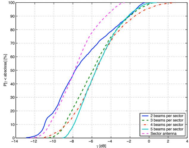
Fig. 4. Expected value of the received common-channel power over the expected value of total interference and noise for a common-channel power of  $P^c=2W$  and a system load corresponding to 95% satisfied users.
