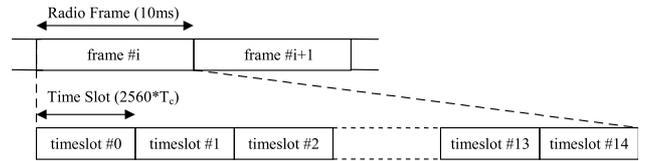
Figure 1. Physical channel signal format [5, 6].
