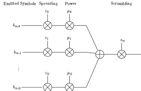
Figure 2. Structure of the UMTS downlink.
