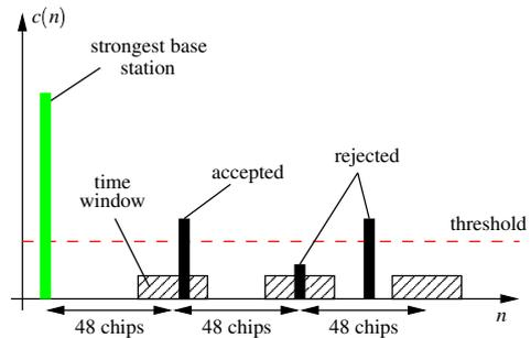
**Figure 5.** Synchronisation to weaker base stations using time windows.
