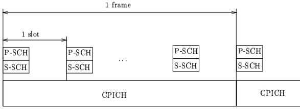
Figure 3. Control channels in FDD.
