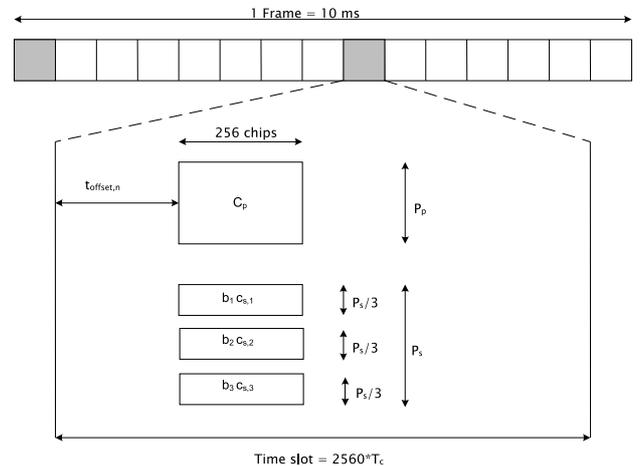
Figure 4. Structure of the TDD synchronisation channel.
