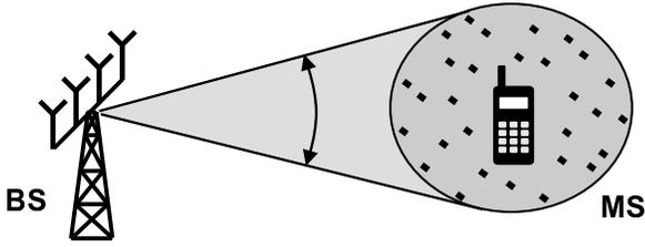
Fig. 1. Visualization of the channel model used for parametrizing the spatial channel properties. The multipath components are inside an angular window, which is centered around the broadside of the base station array.
