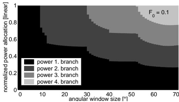
Fig. 5. Optimum power allocation (normalized to the total transmit power) vs. channel parameter for a target outage probability of  $F_0=0.1$ .
