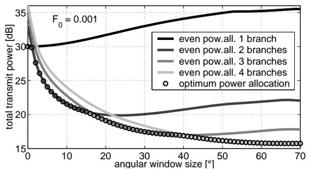
Fig. 6. Required total transmit power vs. channel parameter for a target outage probability of  $F_0 = 0.001$ . Different lines represent different transmit strategies.
