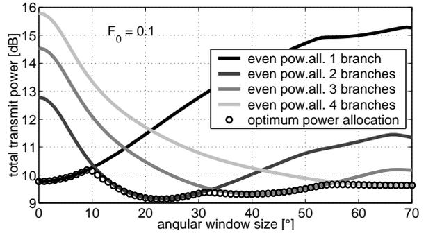
Fig. 3. Required total transmit power vs. channel parameter for a target outage probability of  $F_0=0.1$ . Different lines represent different transmit strategies.
