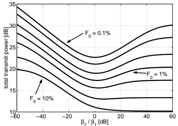
Fig. 9. Required total transmit power vs. power allocation for a system with two correlated diversity branches. Different lines represent different outage probabilities. The outage probability values are (from the bottommost line to the topmost line): 10%, 5%, 2%, 1%, 0.5%, 0.2%, and 0.1%.
