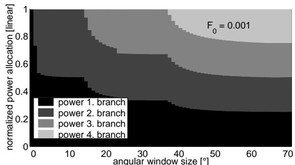
Fig. 7. Optimum power allocation (normalized to the total transmit power) vs. channel parameter for a target outage probability of  $F_0=0.001$ .
