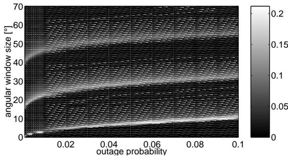
Fig. 8. Performance loss (in terms of additionally required transmit power) of even power allocation compared to optimum power allocation vs. channel parameter and target outage probability.
