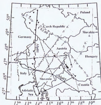
Fig. 2 Field layout of CELEBRATION 2000, 3 rd deployment (grey) and ALP 2002 (black). Shots are shown as triangles, receivers as dots; the lines CEL09 and Alp01 and Alp02 are labeled.
