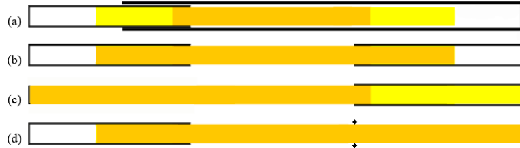
Figure 3.6: Examples of special constellations of PlanningLines: (a) shows overlapping intervals, (b) has no maximum duration, (c) earliest and latest starting-time is the same, (d) missing latest finishing-time in combination with a not defined maximum duration.
