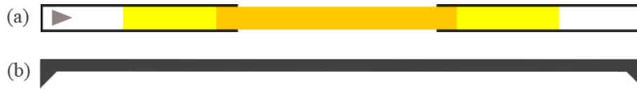
Figure 3.9: Hierarchical decomposition displayed with PlanningLines . (a) shows a collapsed PlanningLine noticeable by the expanding-symbol, (b) shows an expanded PlanningLine as summary bar.
