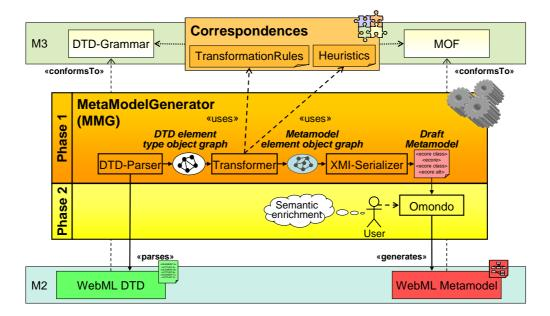
Figure 13: Architecture and Mode of Operation of the MMG
