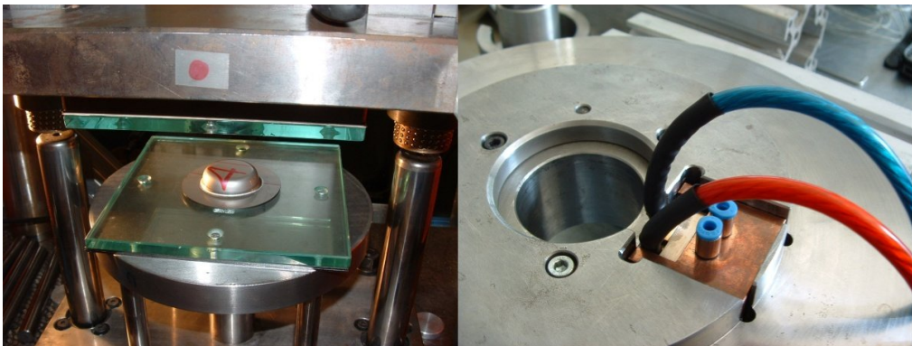
Abbildung 13. Diode Laser installed in a deep drawing tool
