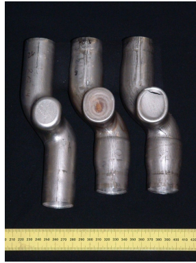
Abbildung 2. Hydroformed Parts starting at the left hand side: After the first forming operation, after the second forming operation with in-between laser treatment, after the second forming operation without laser treatment.
