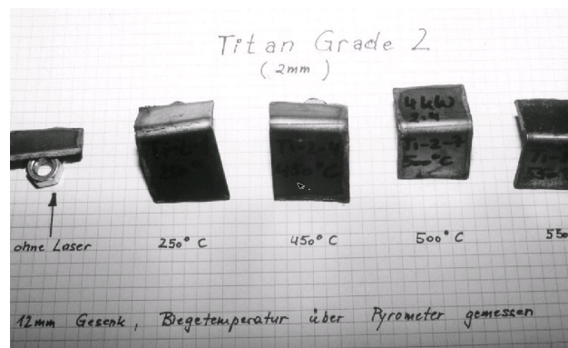
Abbildung 4. Laser assisted Bending: v-shaped die, punch 12
