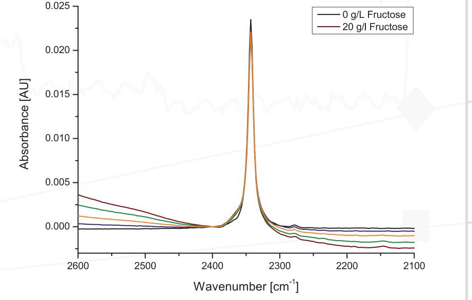
a sample of mineral water was measured. As you can see below the absorbance of CO<sub>2aq</sub> can clearly be seen altough the sampling technique was far from ideal. The spectra also show the most critical problem of the first prototyp. Due to the high power of the globar the spectrometer heats up and the detector signal is drifting.
