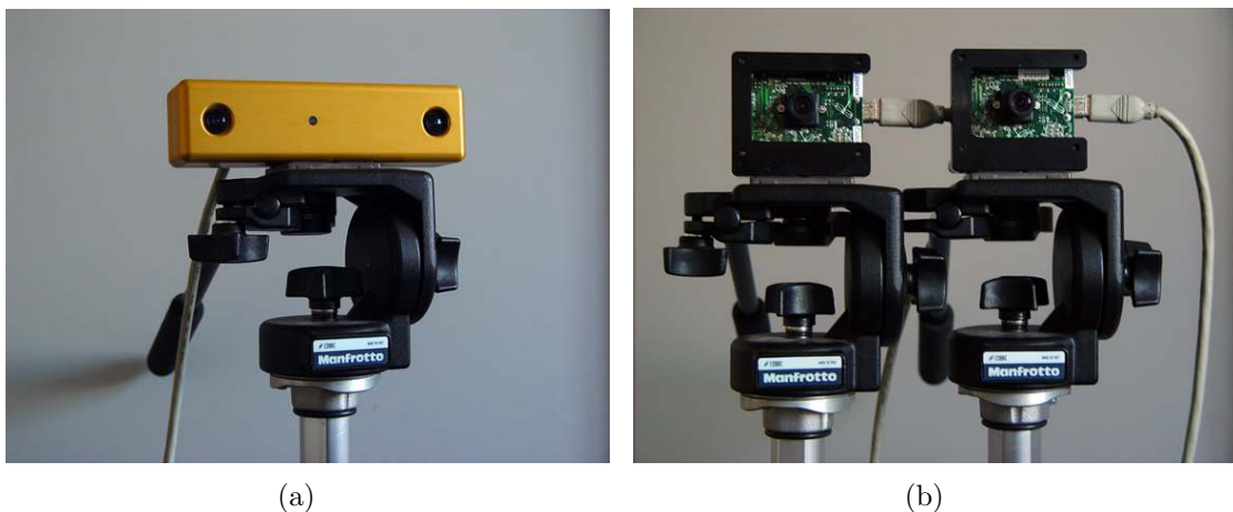
FIGURE 3.3 (a) PointGrey's Bumblebee , a commercially available stereoscopic camera, (b) stereo rig using two PointGrey DragonFly cameras .
