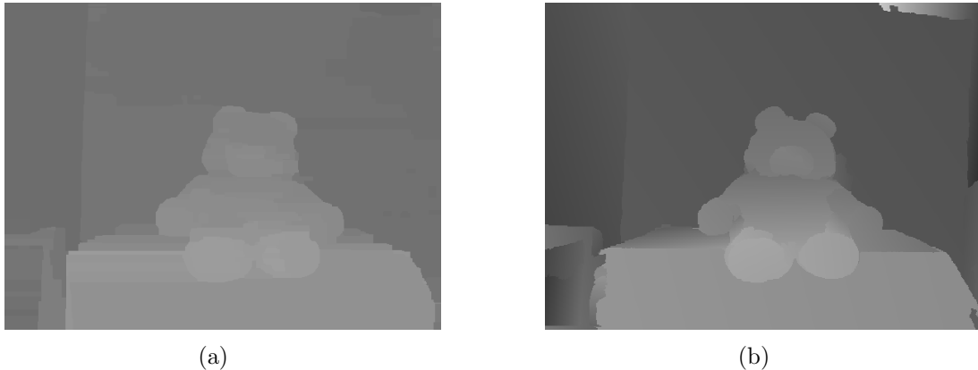
FIGURE 4.4 Disparity maps extracted using (a) Birchfield's and Tomasi's [10] and (b) Bleyer's and Gelautz's [12] methods.
