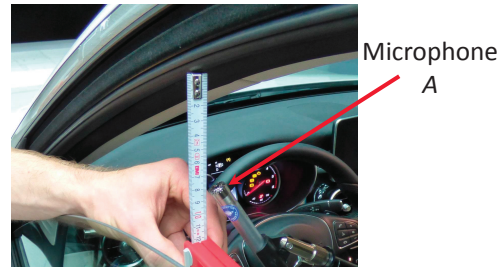
Figure 3: Position of the reference microphone A inside the vehicle.
