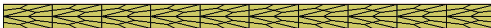
Figure 2: Pseudo one dimensional channel of length L and height H , meshed with strongly distorted elements.
