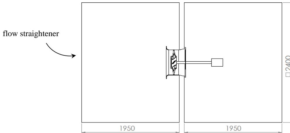
Figure 1 – Geometry of the simulation domain
