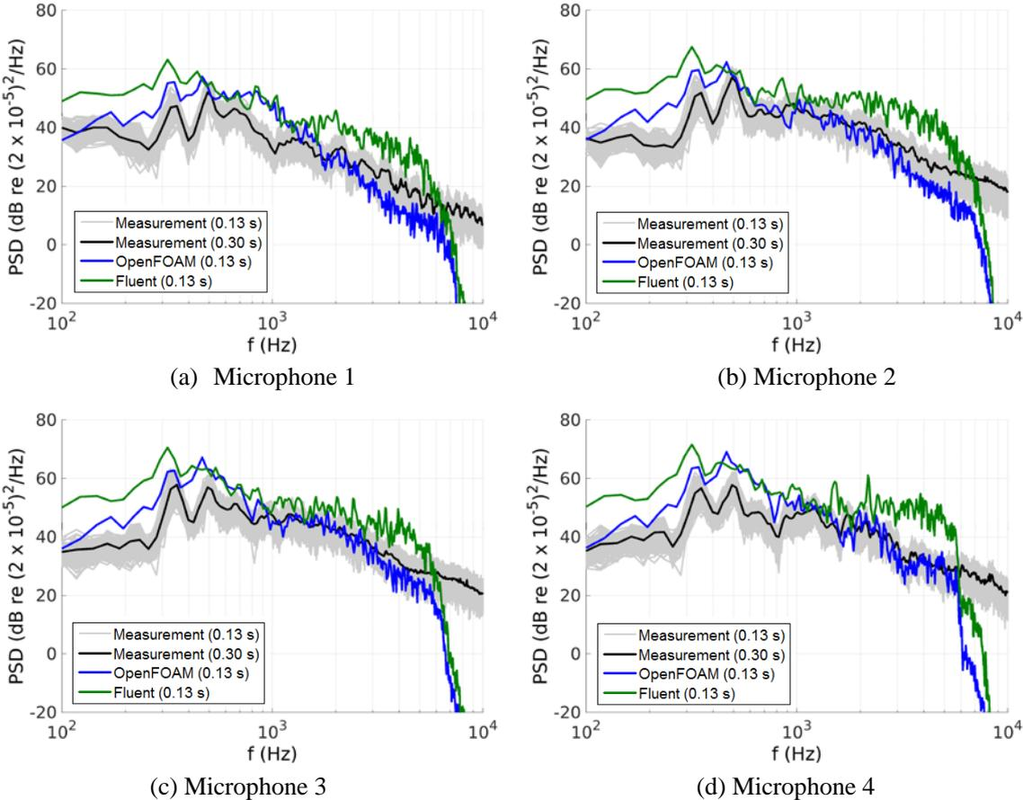
Figure 5 – PSD of the acoustic signal
