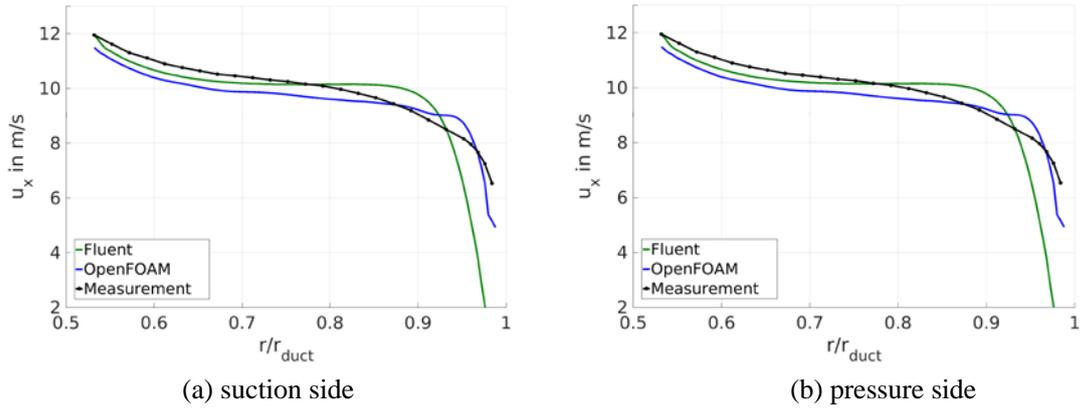
Figure 3 – Time averaged axial velocity
