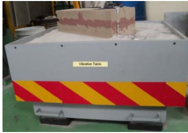
Figure 2. Vibration technique for solidification process
