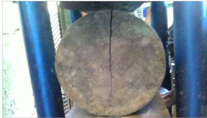
Figure 2. Splitting test set up
