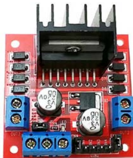
Figure 4. Motor driver L298N
