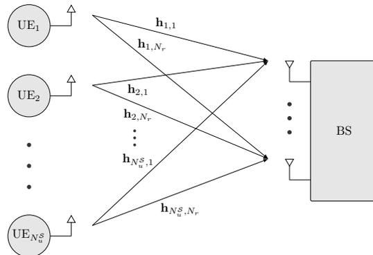
Fig. 1. Illustration of the MIMO MAC for LTE-A uplink.
