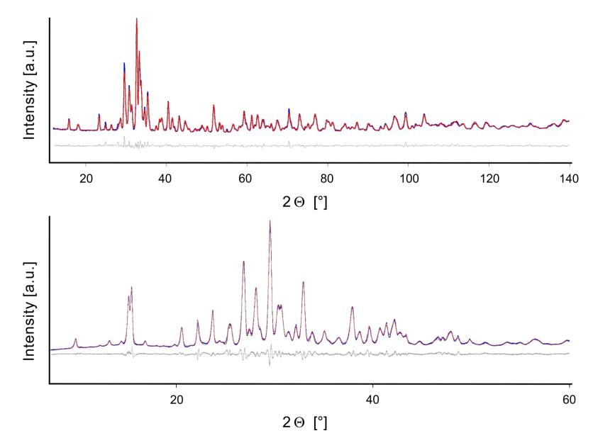
The Diffractograms show the neutron diffraction pattern of alpha NAT on the top and the X-ray diffraction pattern on the bottom. The shown structure is devised of neutron and x-ray diffraction data. Blue dots - nitrogen; Red dots - oxygen; grey dots hydrogen.
