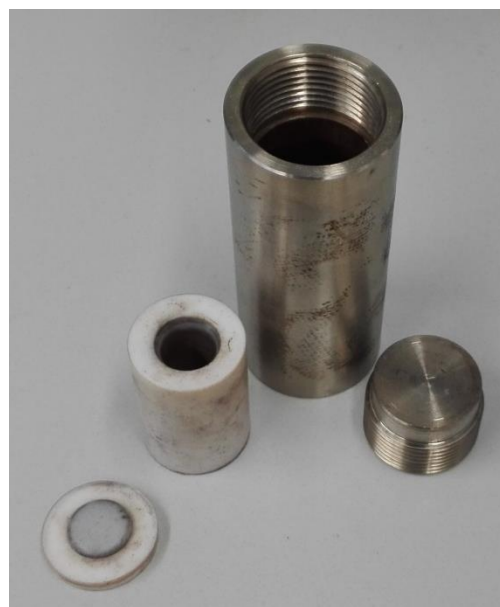
Figure C.01: Teflon®-autoclave (left) with lockable steel jacket (right)
