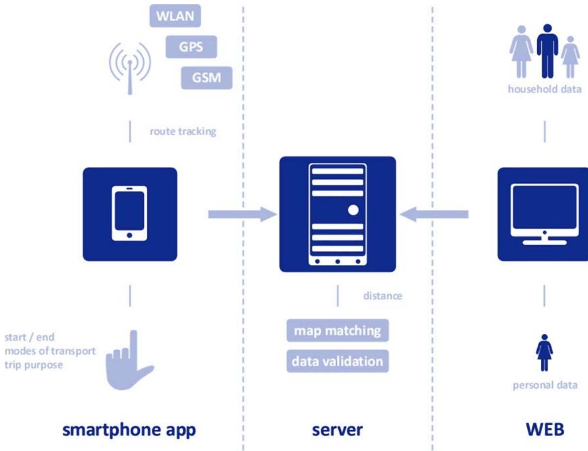
Figure 1. Total system of SmartMo
