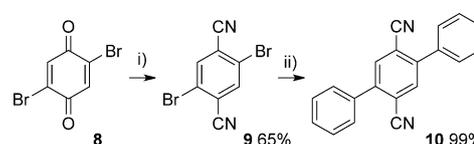
**Scheme 3.** i) Synthesis of 1,4-dibromo-2,5-dicyanobenzene **9** from 2,5-dibromobenzoquinone **8**; conditions: TMSCN, KCN, DMF, 40 min, rt; PBr<sub>3</sub>, MeCN, 1 h, 50 °C; 93 mg. ii) Suzuki coupling of **9** with phenylboronic acid; conditions: [Pd(PPh<sub>3</sub>)<sub>4</sub>], aq. K<sub>2</sub>CO<sub>3</sub>, THF, argon, 6 h, reflux, 69 mg.
