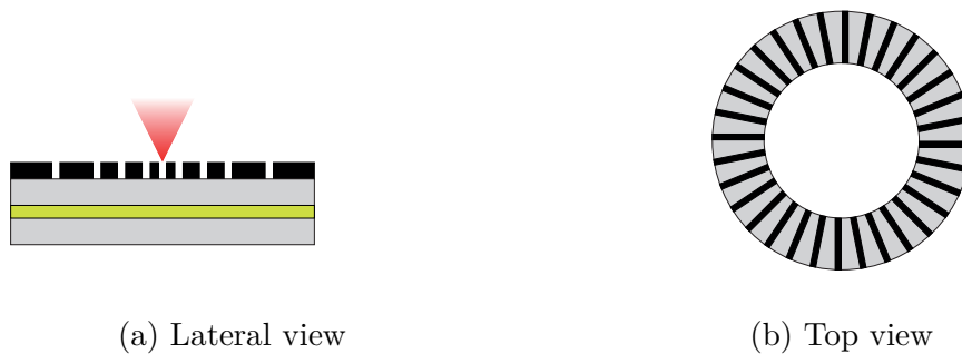
Figure 1.11.: Basic structure of a ring-CSEL. Surface/substrate emission is achieved by a second order grating.
