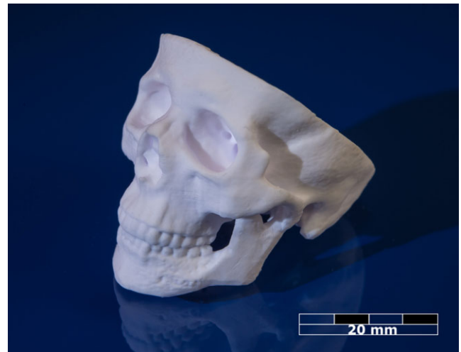
FIGURE 2 Human skull replica made out of tricalcium phosphate (data origin: computer tomography)
