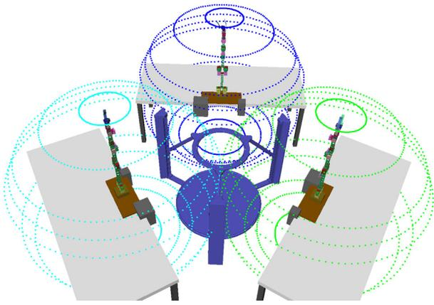
Figure 4: Three robot arms providing 360° haptic coverage.
