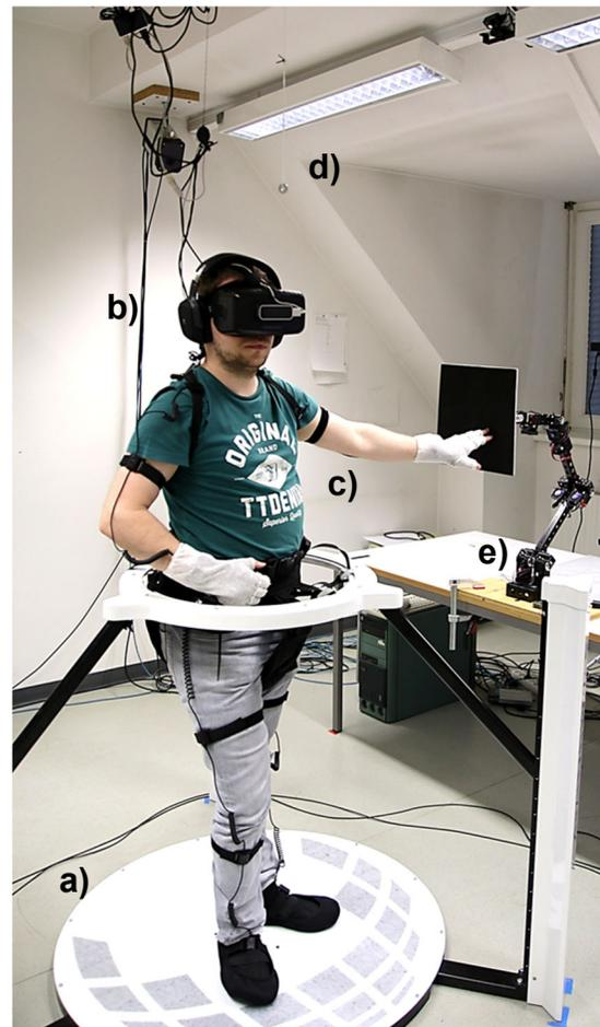
Figure 2: Our fully immersive VR system: a) Cyberith Virtualizer, b) Oculus Rift DK2 with Leap Motion in front and 7.1 audio headset, c) Perception Neuron motion suit with over-gloves, d) perpendicular for initialization, e) Crustcrawler Pro robotic arm.
