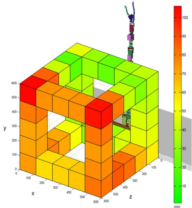
Figure 6: Error map for accuracy in work envelope.
