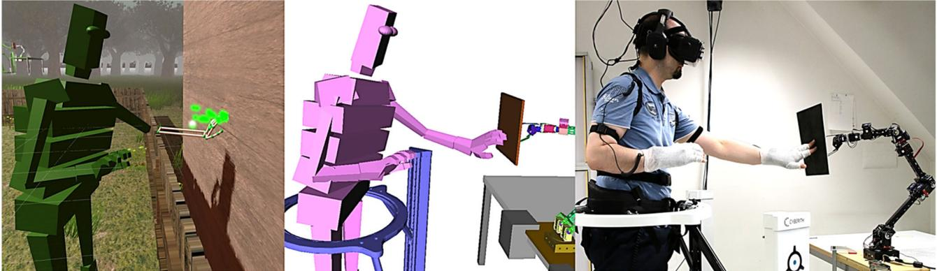
Figure 1: Left: User touches an object in the virtual world. Middle: The correct relative position to the user in the robot environment is known. Right: A physical prop is positioned accordingly in the real world to provide haptic feedback.
