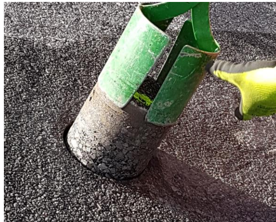
Figure 5. Drill core extraction from an AFRD for bitumen recovery
