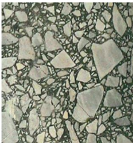
Figure 1. Left: Asphalt matrix (AC 0-11 mm, 6.7 M% Bitumen), Right: Water barrier system of an embankment dam with upstream asphalt concrete facing (AFRD), (ICOLD 1999)
