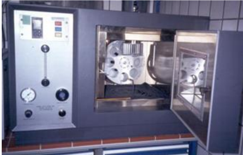
Figure 8. Rolling Thin Film Oven Test
