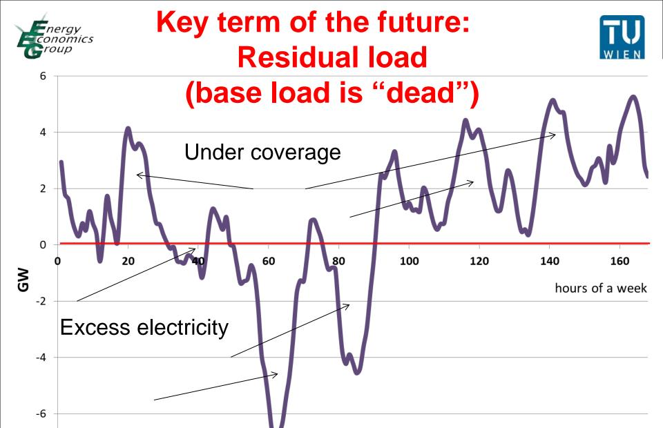
Residual load = Load - non-flexible generation
