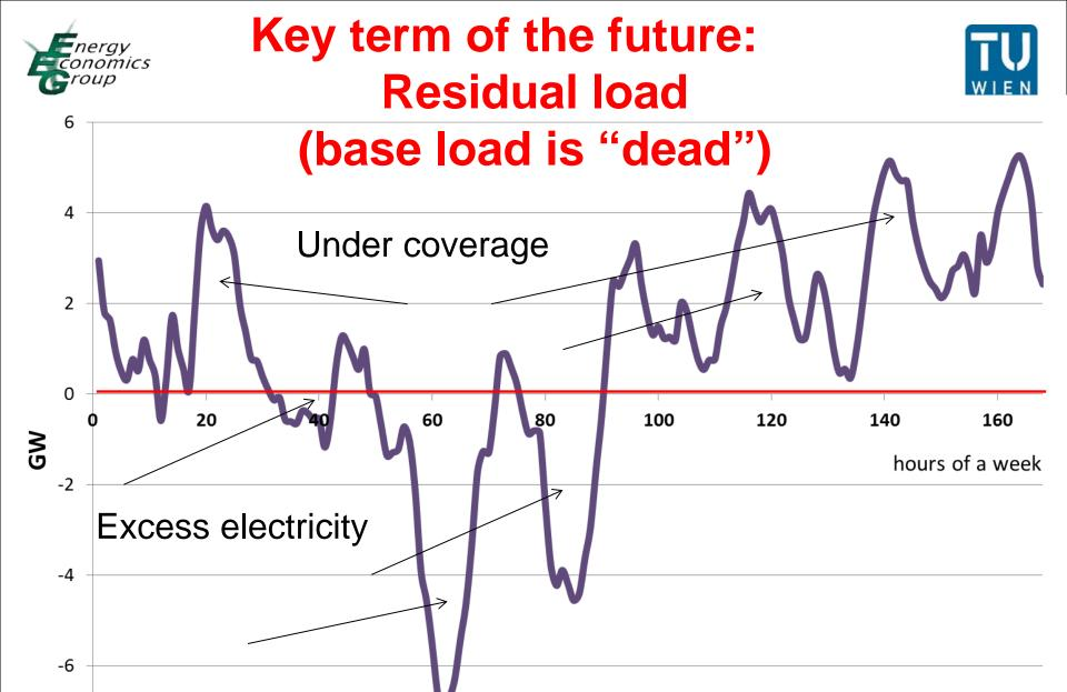
Residual load = Load - non-flexible generation
