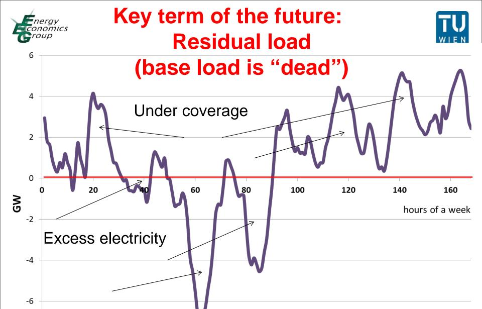
Residual load = Load - non-flexible generation
