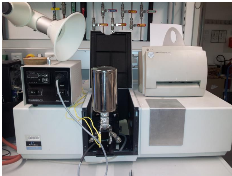
Fig. 1a: UV-VIS-NIR spectroscopy in diffuse reflectance
