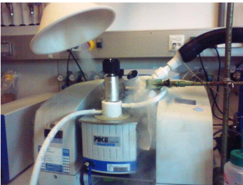
Fig. 2: Variable temperature FIR-MIR spectroscopy in ATR-technique
